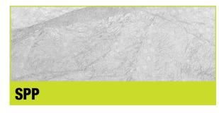
Spunbonded Polypropylene is a lightweight and breathable fabric offering exceptional protection against non-hazardous dry particles. It is an economical solution to protecting workers in dry, dirty environments.
