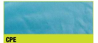
Like Polyethylene, CPE (Chlorinated Polyethylene) is also a polymer, however it is produced through a substitution reaction between polyethylene and chlorine. This reaction gives CPE better water resistance, aging-resistance and chemical-resistance.
